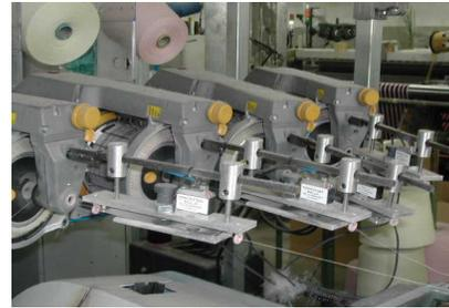
The areas with higher brake effect are during central weft exchange (approx. 150° up to 200° ) and in the weft release (approx. 300° up to 60°)
